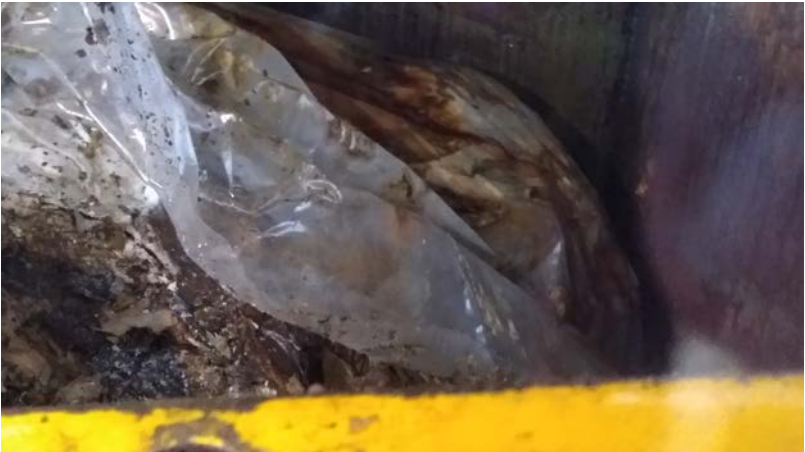
Figure 3 - The paper bale collapsed, reducing the volume by about 30% of the original height. By the touch, the mass appears like moist clay.
